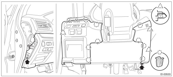
3) Remove the nuts to remove the knee airbag module and disconnect the harness connector. <Ref. to AB-33, KNEE AIRBAG MODULE, PROCEDURE, Airbag Connector.>
