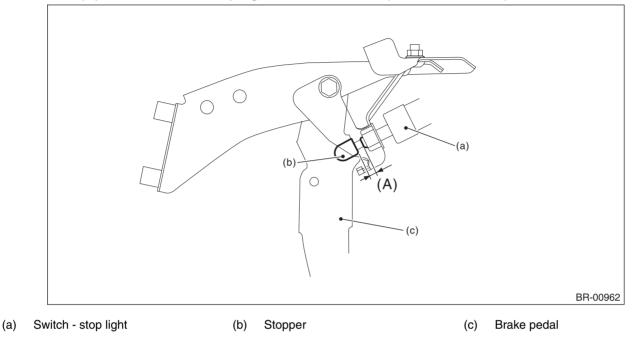
2) Adjust the position of the switch - stop light if the inspection result is not within the standard value. <Ref. to BR-76, ADJUSTMENT, Stop Light Switch.>
