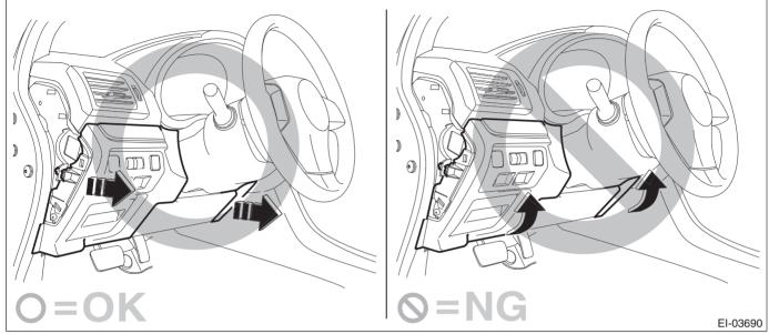
(1) Remove the clips, and remove the cover - instrument panel side LH.
