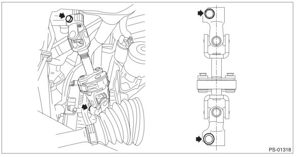
10) Remove the two nuts under the beam COMPL - steering securing the column assembly - steering.
