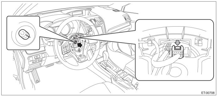
4) Remove the cover assembly - instrument panel LWR driver.
