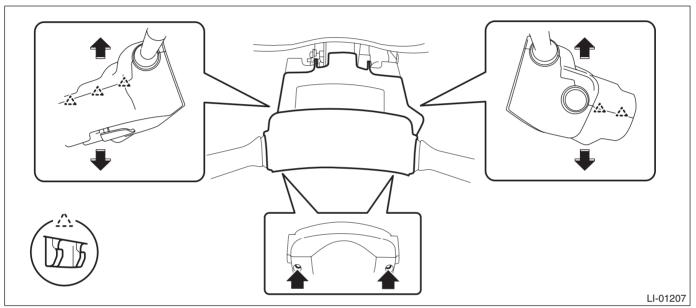
2) Remove the switch assembly - combination.
