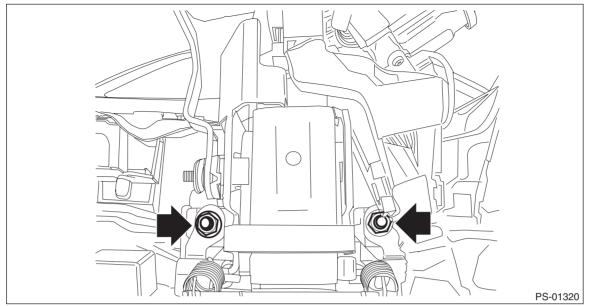
11) Pull out the column assembly - steering from the hole on toe board.
