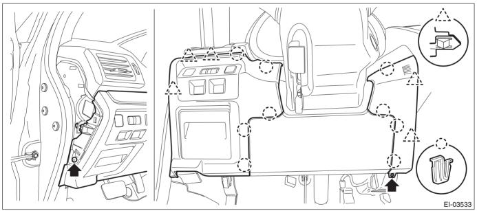
5) Remove the nuts to remove the knee airbag module and disconnect the harness connector. <Ref. to AB-33, KNEE AIRBAG MODULE, PROCEDURE, Airbag Connector.>
