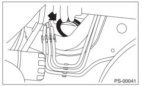
2) Insert the end of the column assembly - steering into the toe board grommet.
