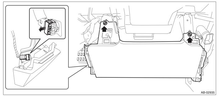
6) Remove the cover assembly - column.
