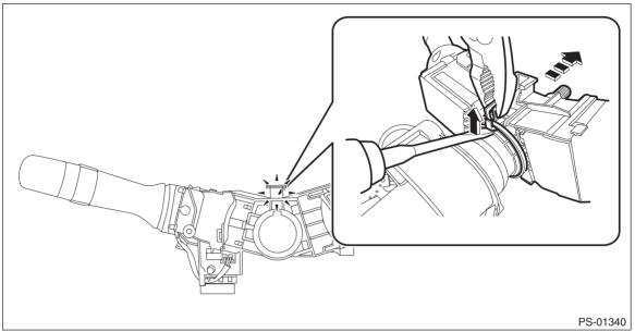
8) Remove all connectors from the column assembly - steering.
