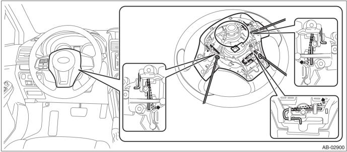
(2) Disconnect the horn harness and airbag connector, and remove the airbag module. <Ref. to AB-24, DRIVER'S AIRBAG MODULE, CURTAIN AIRBAG MODULE & PRETENSIONER, PROCEDURE, Airbag Connector.>
