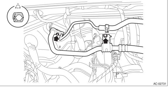
(2) Remove the bolt, and remove the expansion valve - cooling.
