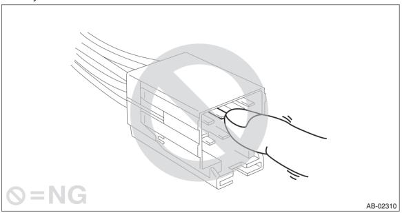
• When checking, use a test harness (1). Damage to connector terminal causes malfunction. Do not directly put the tester probe on airbag connector terminal.
