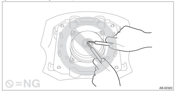
• If damage, open circuit or rust is found on airbag system wiring harness, do not repair the harness. Always replace the faulty harness with a new genuine part.
