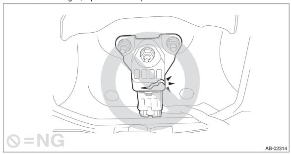
• Install the wiring harness securely with the specified clips to avoid interference or tangled with other parts.
