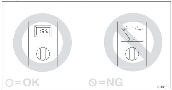
• Do not allow water or oil to come in contact with the connector terminals. Also, do not touch the connector terminals directly.
