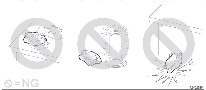
• When storing a removed airbag module, do not place it with the pad side facing downward. Do not place any objects on the airbag module. Do not pile up the airbag module. If the pad of the airbag module is in contact with other objects, it may cause a serious accident if the airbag accidentally operates.
