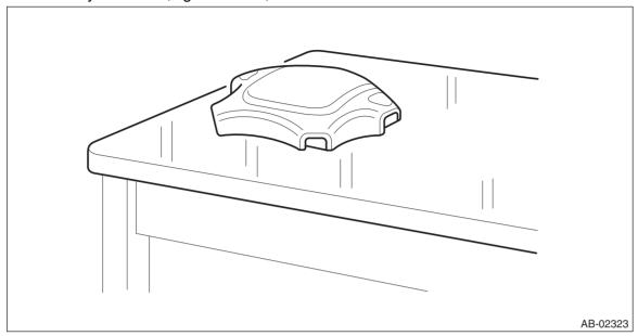
• Do not drop any airbag component, store them under high temperature of 85°C (185°F) or more, or let water, oil or grease get on them; the internal parts may be damaged or the reliability may be greatly lowered.
