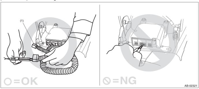
• Do not check continuity of the driver's airbag module, knee airbag module, passenger's airbag module, side airbag module, curtain airbag module or pretensioner.
