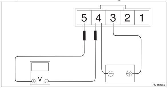
2) Check the voltage changes when air is blown to the mass air flow sensor unit in arrow direction.
