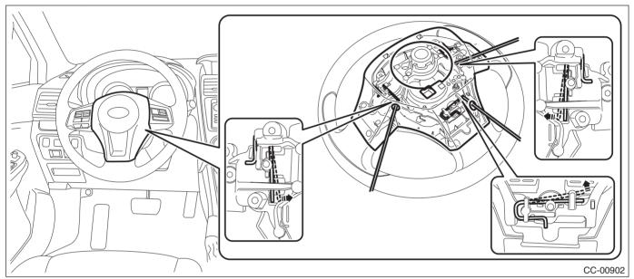
(2) Disconnect the horn harness and airbag connector, and remove the driver's airbag module. <Ref. to AB-24, DRIVER'S AIRBAG MODULE, CURTAIN AIRBAG MODULE & PRETENSIONER, PROCEDURE, Airbag Connector.>
