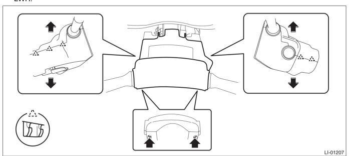
7) Remove the steering roll connector.
