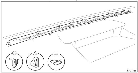
(2) Release the claws, and remove the sensor - automatic light from the panel COMPL - instrument UPR.
