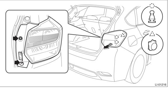
3) Remove the bulb socket and rear side marker light bulb.
