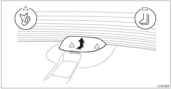
(3) Release the claws and remove the reflector assembly from the light - case.
