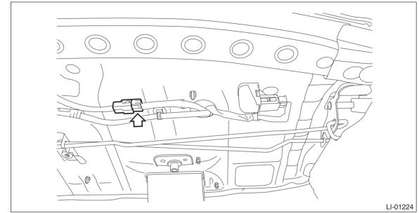
(2) Release the claws, and remove the light assembly - high-mounted.
