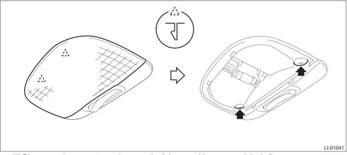
(3) Disconnect the connector and remove the light assembly - room and the bulb.
