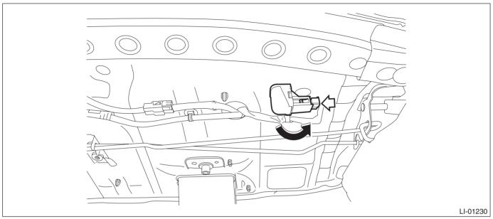
3) Release the claws, and detach the lens and bulb.
