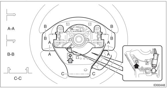
(3) Remove the screws and then remove the satellite switch assembly.
