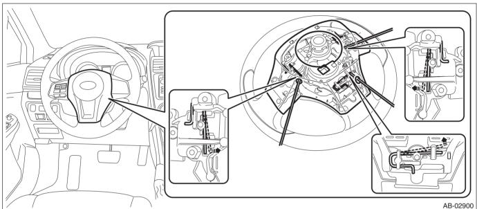
(2) Disconnect the horn harness and airbag connector, and remove the driver's airbag module. <Ref. to AB-20, PROCEDURE, Airbag Connector.>
