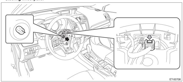
6) Remove the satellite switch assembly.
