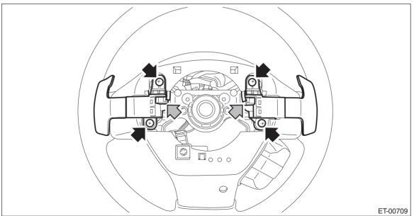
(2) Release the claws and clips, detach the cover - steering wheel LWR.
