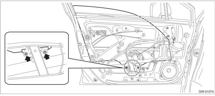
(3) While tilting the glass, remove the glass assembly - front door.
