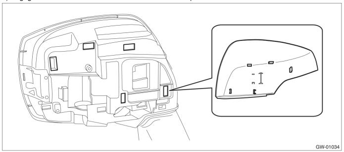
7) Engage the claws into the hole and install the cover - cap outer mirror lower.
