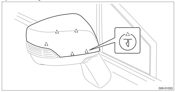
6) Engage the claws into the hole and install the cover - cap outer mirror.
