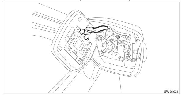
4) Release the claws, and then remove the cover - cap outer mirror lower.
