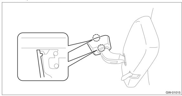
2) Release the lock lever, and slide the mirror assembly - inner rearview to remove.
