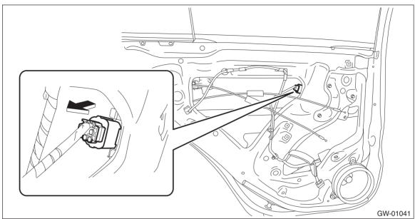
(2) Remove the bolts, and then remove the rear regulator and motor assembly.
