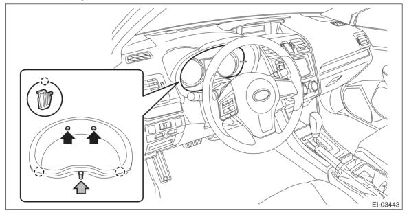
4) Remove the combination meter assembly.
