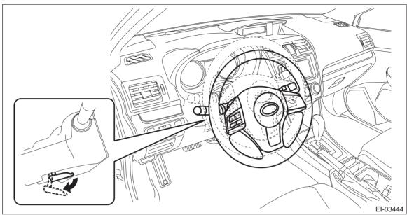
3) Release the screws, clips and claws, and remove the visor - combination meter.
