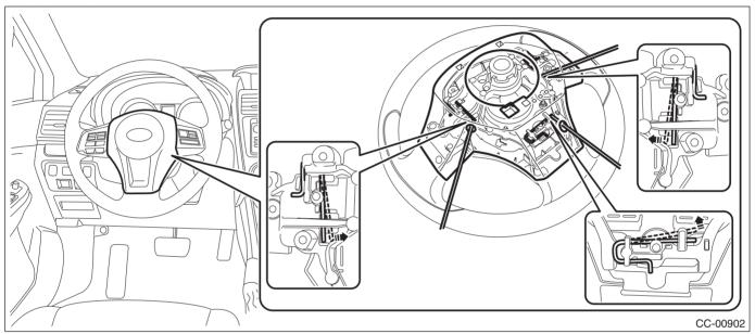
(2) Disconnect the horn harness and airbag connector, and remove the driver's airbag module. <Ref. to AB-20, PROCEDURE, Airbag Connector.>
