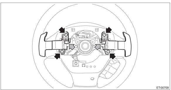
(2) Remove the connector and screw.
