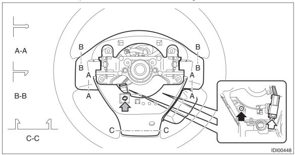
(4) Remove the switch assembly - steering from the cover - steering wheel LWR.
