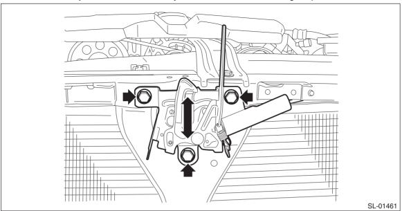
2) After adjustment, tighten the bolts securely.
