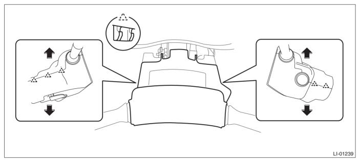
3) Disconnect the connector and remove the immobilizer antenna assembly.
