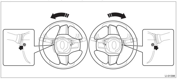
(2) Release the claw, and remove the cover assembly - column UPR and the cover assembly - column LWR.
