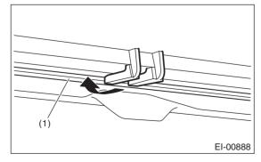
(2) Align the center claw of the cowl panel assembly to the cutout portion of the vehicle side, then install the cowl panel assembly.
