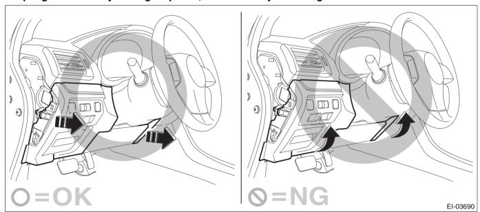
(1) Remove the screws and release the clips and claws.
