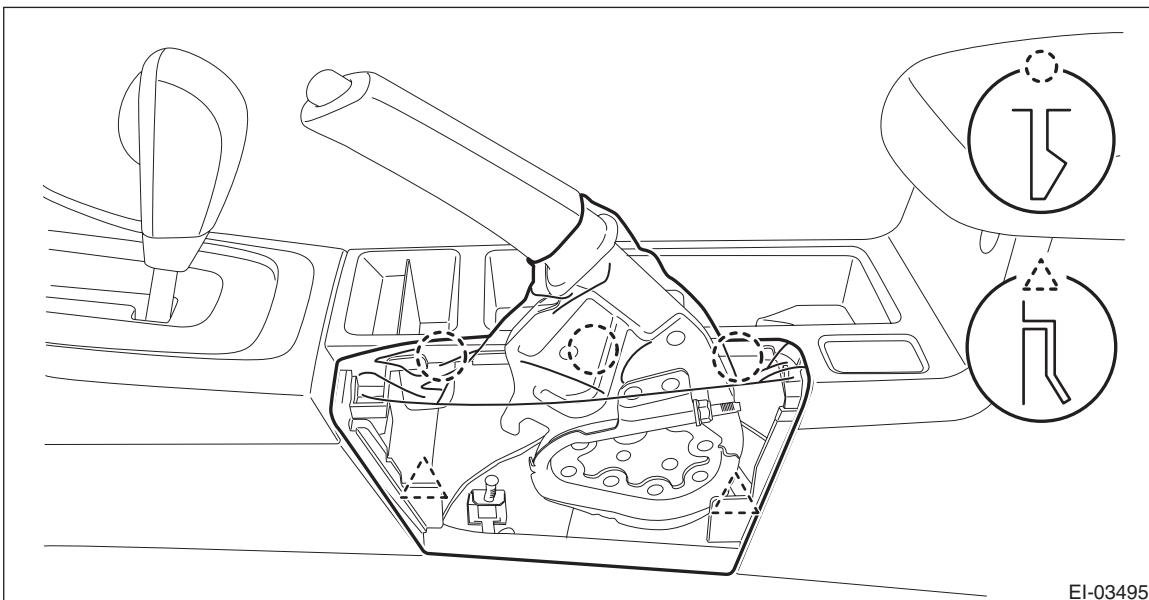
(2) Move the seat forward, and remove the bolts after detaching the left and right caps.
