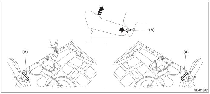
4) Release the clips and claws, and then remove the cover side sill - rear INN.
