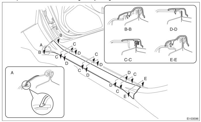
2) Remove the clips, and remove the cover side sill - front.
