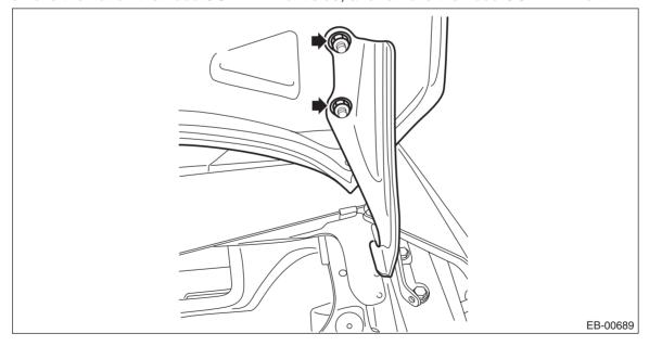
4) Remove the bolts, and remove the hinge COMPL - front hood.
