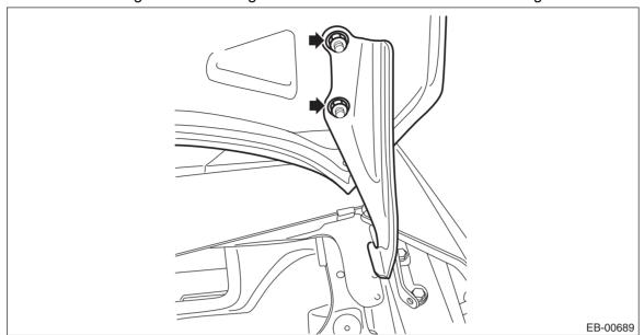
(2) Adjust the horizontal clearance of the hood COMPL - front, and tighten the attaching nuts of the hinge COMPL - front hood.
