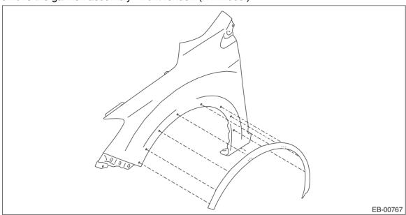
(2) Remove the bolts, and remove the fender COMPL - front.
