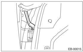
15) Remove the door hinge from vehicle. <Ref. to EB-36, REAR DOOR HINGE, REMOVAL, Rear Door.>
