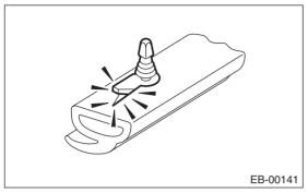
11) Remove the bolts and nuts, and then detach the checker assembly - rear door.
