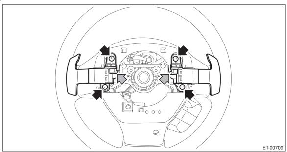
(2) Release the claws and clips, and remove the lower cover - steering wheel LWR.
