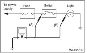
4) With the test set-up held as it is, turn the switch to ON. The voltmeter will indicate a voltage and, at the same time, the light will illuminate.
