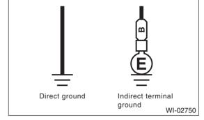
• The ground points shown in the wiring diagram refer to the following:
