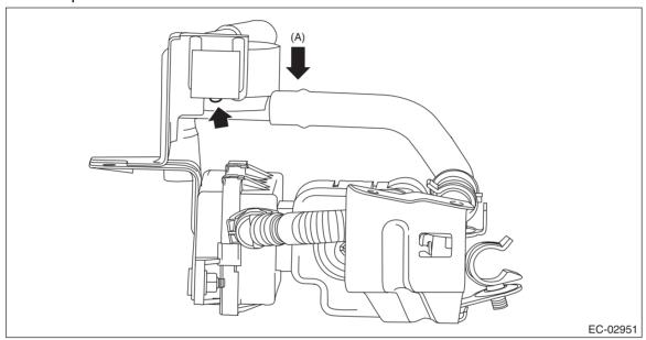
2) Remove the drain hose and drain tube from the drain separator.
