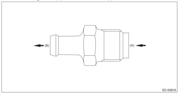
3) Check that air does not come out from (B) when air is blown into (A).
