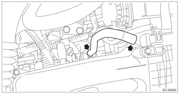
2) Remove the PCV valve from the cylinder block RH.
