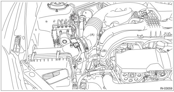
4) Loosen the clamp (A) which connects the air cleaner case (rear) and air intake boot, and then remove the clip (B) from the air cleaner case (front).
