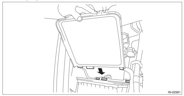
3) Install the clips (B) to the air cleaner case (front), then tighten the clamp (A) that connects the air cleaner case (rear) to the air intake boot.
