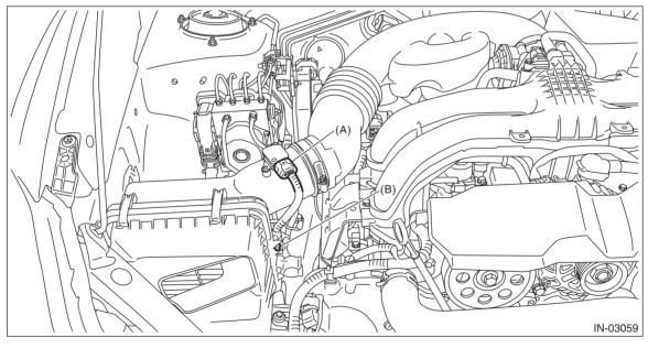
4) Loosen the clamp (A) which connects the air cleaner case (rear) and air intake boot, and then remove the clip (B) from the air cleaner case (front).
