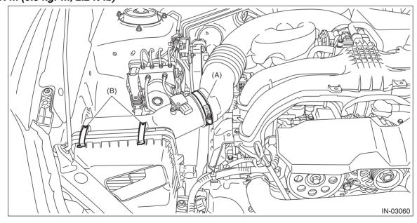
4) Connect the connector (A) to the mass air flow and intake air temperature sensor and secure the harness with clip (B).
