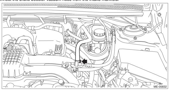
3) Connect the vacuum gauge to the intake manifold.
