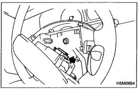
5) Disconnect airbag connector on back of airbag module. < Ref. to 5-5 [M2-6].☆1>
