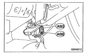
3) Remove lower cover. < Ref. to 5-4 [W1A0].☆1> Disconnect airbag connector (AB3) and (AB8) below steering column.
