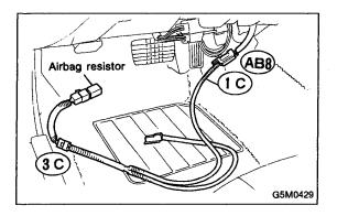
10) Turn ignition switch "OFF", disconnect battery ground cable, and wait 20 seconds. Remove lower cover panel and connect test harness C connector (1C) to (AB8) < Ref. to 5-4 [W1A0].☆1 > with airbag resistor attached to test harness C connector (3C).
