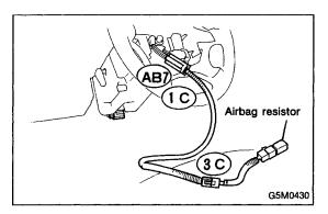
8) Turn ignition switch "OFF", disconnect battery ground cable, and wait 20 seconds. Connect connector (AB8) to (AB3). Remove driver side airbag module and connect test harness C connector (1C) to (AB7). <Ref. to 5-5 [W3A1].☆1>
