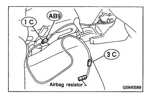
11) Turn ignition switch "OFF", disconnect battery ground cable, and wait 20 seconds. Disconnect passenger side airbag module connector (AB9) to (AB10). < Ref. to 5-5 [W3A2].☆1>
