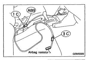
6) Turn ignition switch "OFF", disconnect battery ground cable, and wait 20 seconds. Disconnect passenger side airbag module connector (AB9) to (AB10). <Ref. to 5-5 [W3A2].☆1> Connect test harness C connector (1C) to (AB9).
