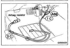
7) Turn ignition switch "OFF", disconnect battery ground cable, and wait 20 seconds. Connect passenger side airbag module connector (AB9) to (AB10). Connect battery ground cable and turn ignition switch "ON". Does airbag warning light go "OFF" after 8 seconds and remain off for more than 30 seconds?
