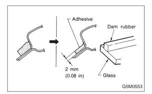
2) Finishing adhesion surface on body side Using a cutter knife etc., cut layer of adhesive sticking firmly to body, and finish it to a smooth surface of about 2 mm (0.08 in) in thickness.
