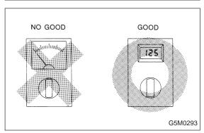
3) When checking the system, be sure to use a digital circuit tester. Use of an analog circuit tester may cause the airbag to activate erroneously. Do not directly apply the tester probe to any connector terminal of the airbag. When checking, use a test harness.
