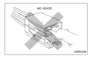
8) Do not allow water or oil to come in contact with the connector terminals. Do not touch the connector terminals.
