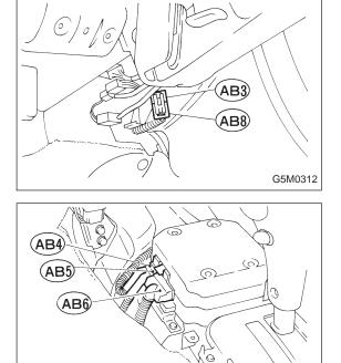
3) Remove lower cover. <Ref. to 5-4 [W1A0].> Disconnect airbag connector (AB3) and (AB8) below steering column.
