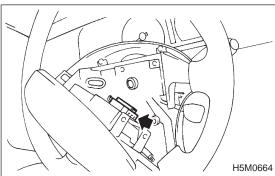
5) Disconnect airbag connector on back of airbag module. <Ref. to 5-5 [M2-6].>
