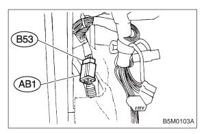
5) Disconnect body harness connector (B53) from connector (AB1).
