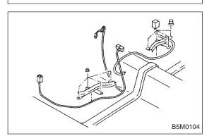
7) Roll up floor mat and side sill lower cover of both side and then remove main harness.
