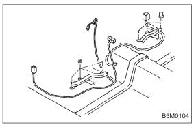
7) Roll up floor mat and side sill lower cover of both side and then remove main harness.
