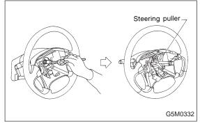
7) Using steering puller, remove steering wheel.
