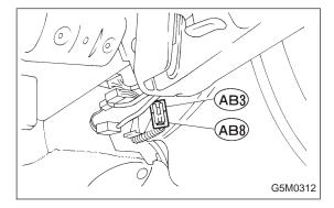
3) Remove lower cover. <Ref. to 5-4 [W1A0].> Disconnect airbag connector (AB3) and (AB8) below steering column.
