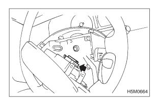
6) Disconnect airbag connector on back of airbag module. <Ref. to 5-5 [M2-6].> Remove airbag module, and place it with pad side facing upward. <Ref. to 5-5b [W300].>
