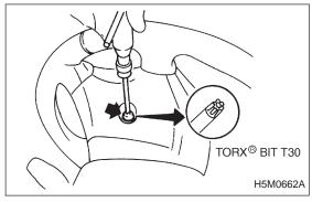
4) Using TORX® BIT T30, remove two TORX® bolts.
