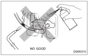
When painting or performing sheet metal work on the front part of vehicle body, including the front wheel apron, front fender and front side frame, take utmost care not to apply dryer heat, painting mist, or the flame of the welding burner directly to the front sensors and wire harness of the airbag system.
