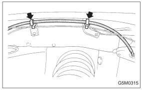
8) Remove wiring harness clips.
