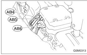
4) Remove console box. <Ref. to 5-4 [W1A0].> Disconnect 2-pin blue connector (AB4) (right side front sensor) and 2-pin orange connector (AB5) (left side front sensor) from airbag control module. <Ref. to 5-5 [M2-6].>
