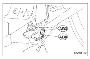
3) Remove lower cover. <Ref. to 5-4 [W1A0].> Disconnect airbag connector (AB3) and (AB8) below steering column.
