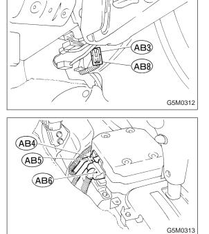
3) Remove lower cover. <Ref. to 5-4 [W1A0].> Disconnect airbag connector (AB3) and (AB8) below steering column.
