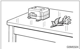
• After removal, keep the airbag control module on a dry, clean surface away from heat and light sources, and moisture and dust.
