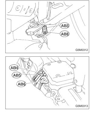
3) Remove lower cover. <Ref. to 5-4 [W1A0].> Disconnect airbag connector (AB3) and (AB8) below steering column.
