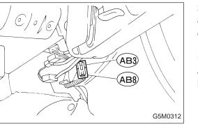
3) Remove lower cover. <Ref. to 5-4 [W1A0].> Disconnect airbag connector (AB3) and (AB8) below steering column. **CAUTION:**
