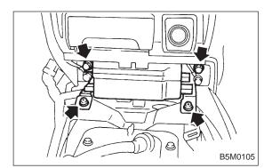
6) Using TORX<sup>®</sup> BIT T40 (Tamper resistant type), remove two TORX<sup>®</sup> bolts.
