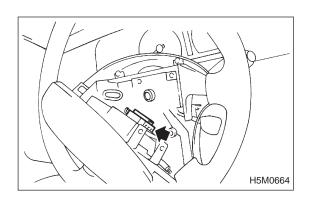
6) Disconnect airbag connector on back of airbag module. <Ref. to 5-5 [M2-6].> Remove airbag module, and place it with pad side facing upward. <Ref. to 5-5 [W300].>
