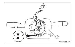
3) Then, back off roll connector pin ① approximately 2.65 turns until "▲" marks aligned.
