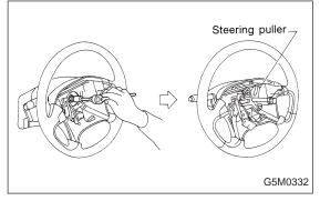
7) Using steering puller, remove steering wheel.
