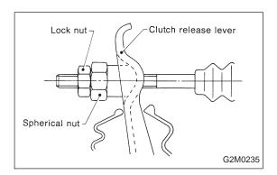
3) Upon completion of adjustment, securely lock spherical nut with lock nut.
