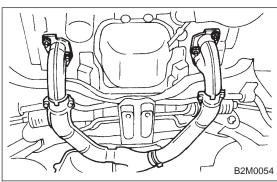
6) Remove bolts which hold front exhaust pipe onto cylinder heads.
