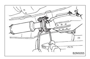
4) Install center exhaust pipe to rear exhaust pipe.
