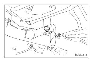
7) Remove front exhaust pipe and center exhaust pipe from hanger bracket.
