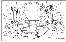
3) Tighten bolts which hold front exhaust pipe onto cylinder heads.
