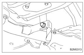
2) Install front exhaust pipe and center exhaust pipe. And temporarily tighten bolt which installs center exhaust pipe to hanger bracket.
