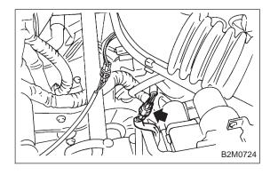
9) Connect front oxygen sensor connector.
