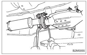
5) Separate center exhaust pipe from rear exhaust pipe.
