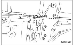
6) Connect rear oxygen sensor connector. (Except California 2200 cc model)
