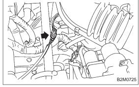
2) Disconnect rear oxygen sensor connector. (California 2200 cc model)
