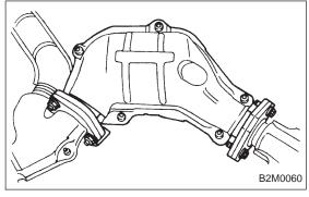
8) Separate front catalytic converter from front exhaust pipe and center exhaust pipe.
